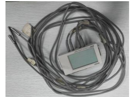
Thermocouple sensor and 4 channel data recorder
